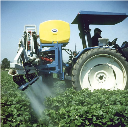
ESS air-assisted electrostatic sprayers allow you to cover an average of 30 or more acres per 150 gallon tank of chemical. Compare this to the 500 gallon tank on most hydraulic
